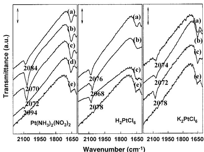
Fig. 3. FT-IR spectra of adsorbed CO on 0.5 wt.% Pt/ $\gamma$ -Al<sub>2</sub>O<sub>3</sub> catalysts after calcination at different temperatures and reduction at 573 K. (a) Calcination  $T = 373$  K, (b) calcination  $T = 573$  K, (c) calcination  $T = 773$  K, (d) calcination  $T = 1073$  K and (e)  $\gamma$ -Al<sub>2</sub>O<sub>3</sub> support. CO molecules were adsorbed at RT for 1 h and evacuated at the same temperature for 0.5 h.
