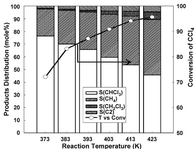
Fig. 1. Effects of reaction temperature on HDC of  $\text{CCl}_4$  by using 0.5 wt.%  $\text{Pt}/\gamma\text{-Al}_2\text{O}_3$  catalyst prepared from  $\text{Pt}(\text{NH}_3)_2(\text{NO}_2)_2$ . Catalyst (0.5 g) was reduced at 573 K after drying at 373 K.  $P_g = 0$  bar, WHSV = 9000 l/(kg h),  $\text{H}_2/\text{CCl}_4 = 9$ .
