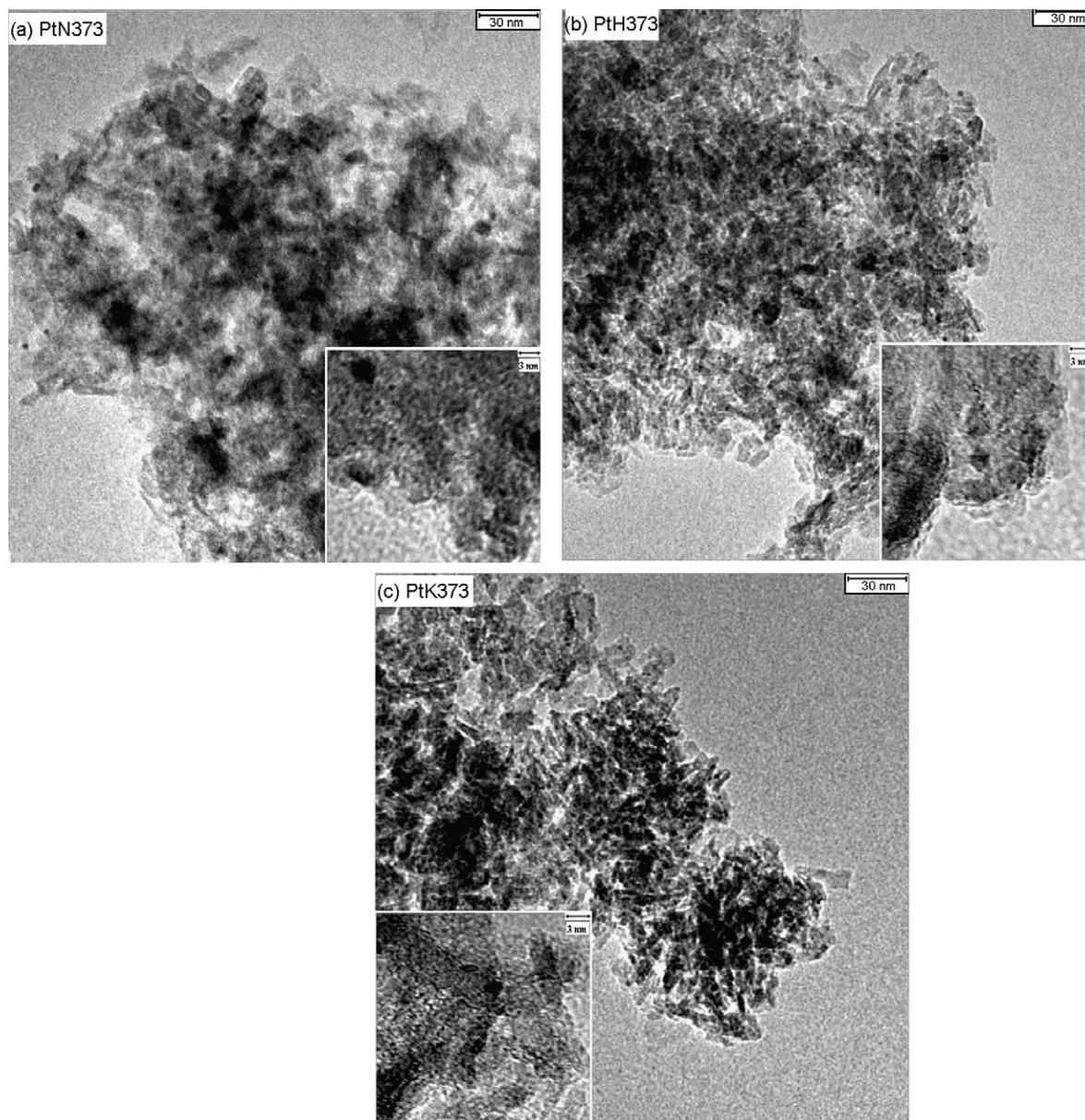
Fig. 2. HRTEM images of 0.5 wt.% Pt/ $\gamma$ -Al<sub>2</sub>O<sub>3</sub> catalysts prepared from different platinum precursors after drying at 373 K and reduced at 573 K. (a) PtN373, (b) PtH373 and (c) PtK373.
